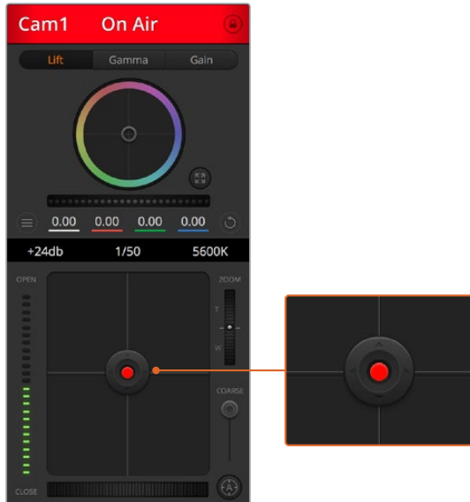
The iris/pedestal control illuminates red when its respective camera is on air.
